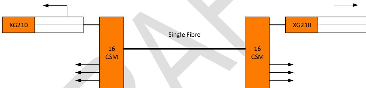
Each Service design can support up to a maximum of three ADVA XG210 units per filter endpoint with each XG210 pairing being able to support up to two 10Gbps customer services. Each 10Gbps circuit uses a wavelength port on the filter. Fully deployed as above there would be 10 spare wavelength ports on the filter set.
