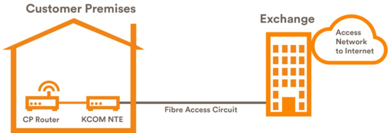
Wholesale DIA circuits provide an adaptable dedicated link to the Internet, they provide a high-speed Internet connection for a company’s Local Area Network (LAN). Service options range from 10Mbps to 10Gbps, providing dedicated access with a high-speed “always-on” connection.
